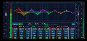
Picture above shows a 10 band graphic EQ, as you can see it adjusts adjacent frequencies as well, 30 band does the same with just less width
