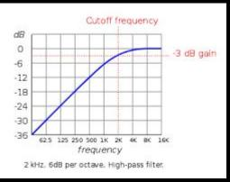
Left shows a 2khz, 6dB per octave high-pass(low cut) filter
